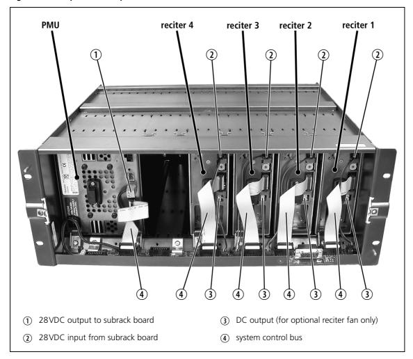
The TB8100 subrack can accommodate one to seven reciters, or one to five reciters with a PMU (as shown in Figure 7). When fitted, the PMU occupies reciter positions 6 and 7 (numbered from right to left viewed from the front).
